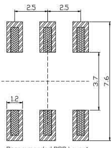
Recommended PCB Layout Top View
