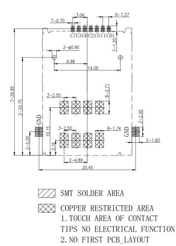
CIRCUITS IN THE AREA Recommended PCB Layout
