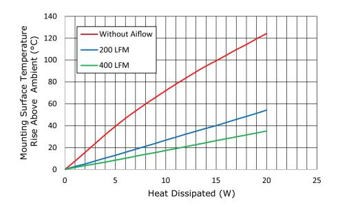
Ths: "hot spot" temperature measured on the heatsink
