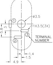
Recommended PCB Layout Top View
