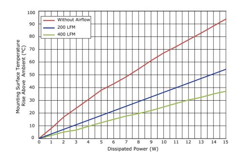
Ths: "hot spot" temperature measured on the heatsink Ta: ambient temperature
