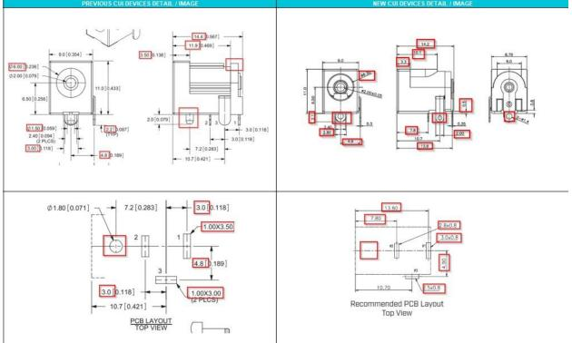
Description of Change: Mechanical, electrical, and material changes as shown below:
