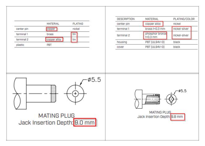
Insertion/extraction force adjusted to 0.3 ~ 2.0 kg
