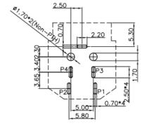
Recommended PCB Layout Top View
