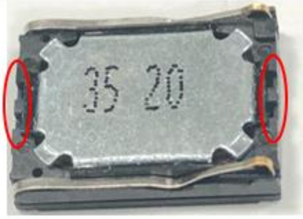
With notches on new plastic housing.
