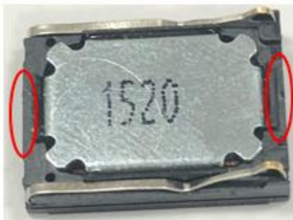
Without notches on old plastic housing.
