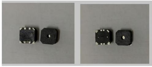
The only change is the injection Molding. This does not change any of the Characteristics of the product.
